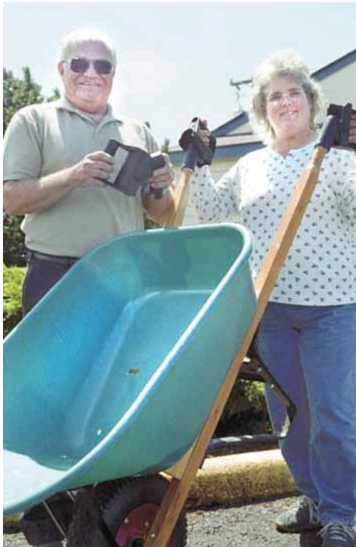
Suzanne and Mel Lulay of Waldport demonstration how their Simply Dump It wheelbarrow handles work. The handles slip on the wheelbarrow and are secured by a screw. Plastic shims come with the handles so they can be adjusted to fit different sizes of handles. A pivot-point allows for the user to dump the wheelbarrow without losing control of the wheelbarrow's load. The Lulays are from Waldport and plans to show their invention at the Lincoln County Fair, July 15 to 18. (Photo by Susan T. Wehren)
